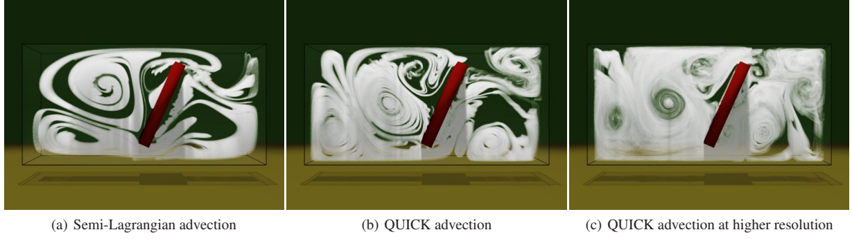
Figure 2: Smoke stirred by a paddle. Panel (a) is produced using semi-Lagrangian advection on a 64 \times 32 \times 32 grid. The large amount of numerical viscosity suppresses the naturally occurring unstable motions in the flow, leading to a smoke field that is highly filamented but without smaller scales in the flow. Panels (b) and (c) are produced using QUICK advection on grids of the same and higher resolution ( 128 \times 64 \times 64 ) respectively. Especially in panel (c), natural instabilities are no longer suppressed and the flow field exhibits a naturally turbulent field containing many scales.
