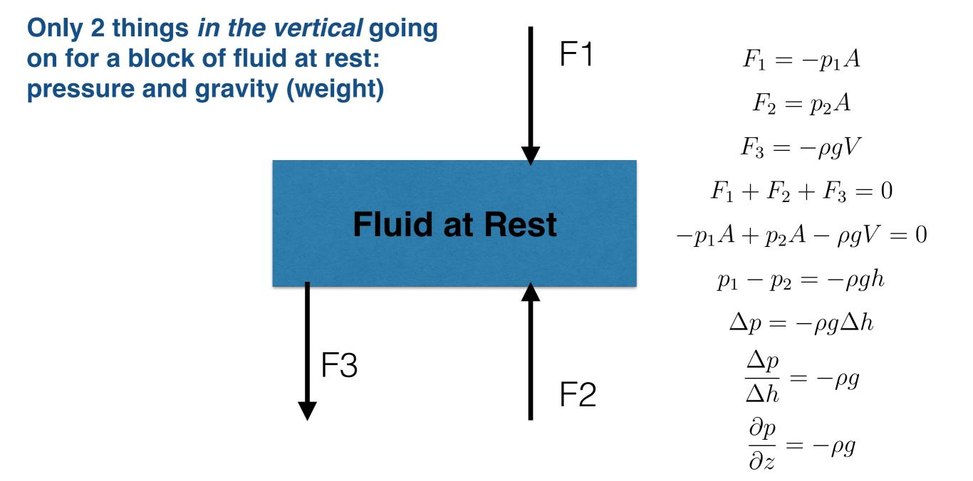
Hydrostatic balance just says that at any point in the water column, the pressure is proportional the weight of the fluid above it. So at larger depth, the pressure is larger
