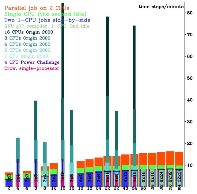
Same as before, but showing cases with up to 16 Origin 2000 CPUs involved: the code scales perfectly to this number of processors and it is clear that it is vector length which matters most for Origin 2000
