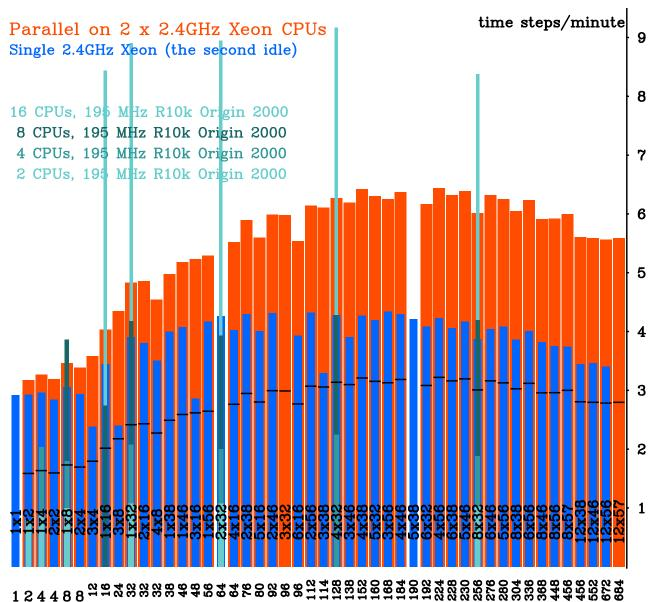
Performance 1/2 degree,  $384 \times 224 \times 32$  grid Pacific model on dual 2.4 GHz Xeon machine: Overall, with proper choice of partitions the dual Xeon machine runs as fast as to 12 195MHz R10k CPUs of Origin 2000. It takes 10 hours of computing (wall clock) to get one model year of simulation, which makes it viable choice (time step 7200 sec; mode splitting ratio ndtfast=78; FB barotropic mode).
