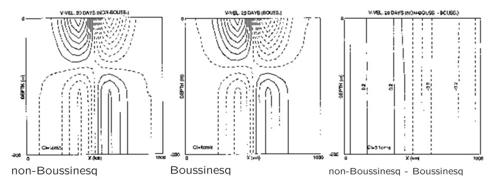
Field shown: tangential velocity component; contour interval 1cm for 2 left panels; 0.1 for difference. Max value 7cm/sec near surface; 3.5 near bottom.
