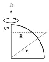
Figure 2: Vectors indicating position  $(\vec{r})$  and distance from spin axis  $(\vec{R})$  extending to the location shown.
